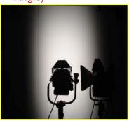
The Barndoor in a NOT REAL FRESNEL optics does not work properly: the projection is OVAL and the more you barndoor the more you dim the central beam
