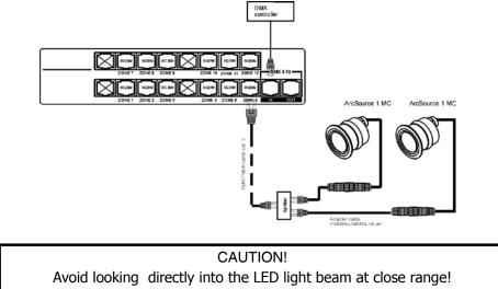
Connect the ArcSource 1 MC to the driver via the adapter cable Chogori/RJ45 and use suitable cable joint box (weather-tight for outdoor installation) if the cable has to be extended. Use a cable splitter if more than one LED module has to be connected to the one LED output of the driver, the connection between the ArcPower and the splitter is a standard RJ45 patch cable category 5 wired 1:1.
