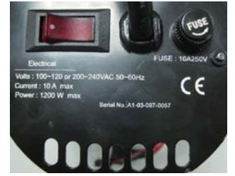
On/Off switch, universal 100-240V power input and fuse protection
