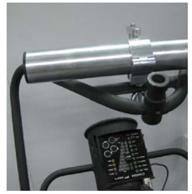
Rigging on truss through the 13mm hole in the center of the bracket plate
