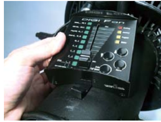
Switch for local or DMX operation mode
