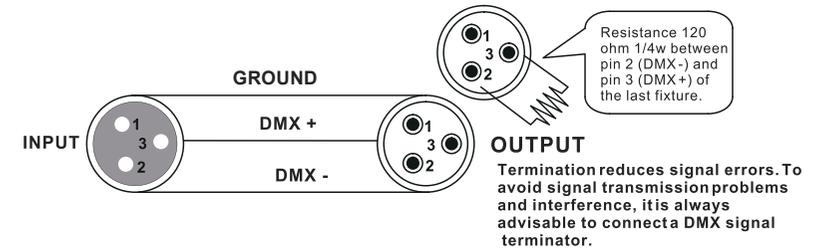
caution: Do not allow contact between the ground and the fixture's chassis ground. Grounding the ground can cause a ground loop, and your fixture may perform erratically. Test cables with an ohm meter to verify positive pole and to make sure the pins are not grounded or shorted to the shield or each other.
