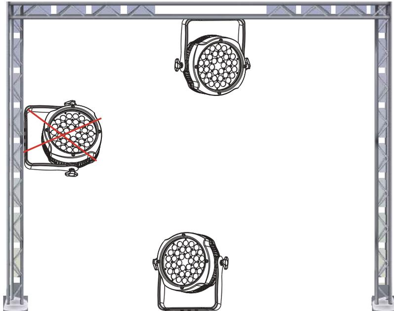
The AT-PPL-UV is fully operational in two different mounting positions, hanging upside-down from a ceiling or set on a flat level surface. To avoid internal damage to the unit, never mount the unit on its side as illustrated above. Be sure this fixture is kept at least 0.5m away from any flammable materials (decoration etc.). And you'd better use and install the supplied safety cable as a safety measure to prevent accidental damage and/or injury in the event the clamp fails (see next page).
