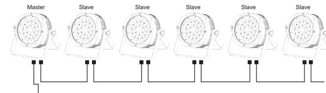
First, set one light, which involves the program you have edited in EDIT menu and want to upload, in Master mode, and others in Slave mode. Then, connect all the lights with DMX cables. Finally, select the UPLOAD menu of the Master light and press ENTER. All the programs edited in the Master light will be uploaded to the Slave lights.
